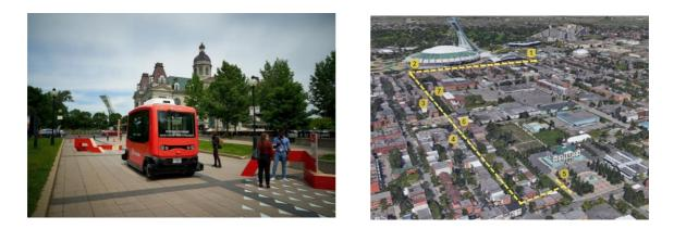
In this project, Transdev operates two EasyMile autonomous shuttles that circulate in the normal daily traffic conditions, crossing intersections equipped with intelligent traffic signals with which the shuttles communicate, thus providing a new transport service, useful to the inhabitants of Montreal, between the Olympic Park and the Maisonneuve Market.
