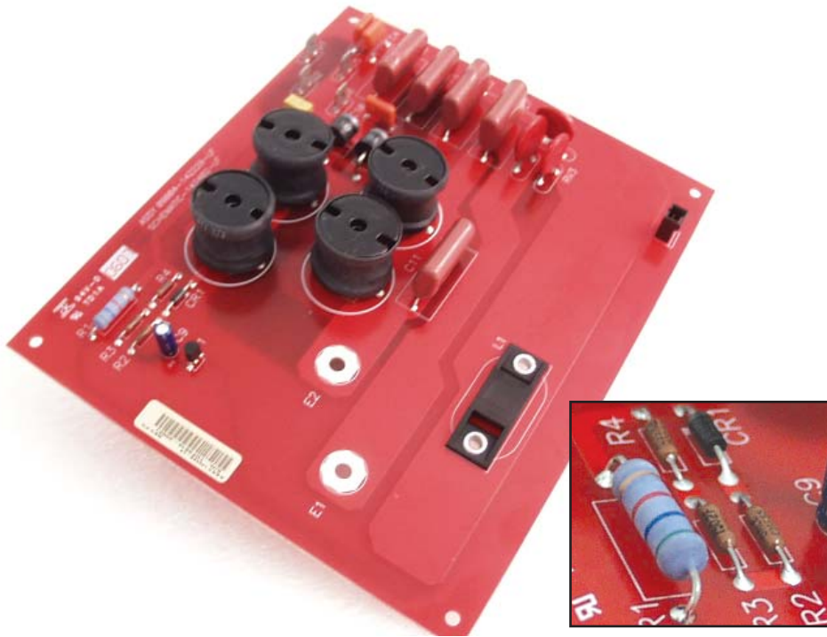
Figure 6: Printed Circuit Assembly color coded "Red", signifying Lead Free and utilizing Tin-Copper-Nickel Alloy
