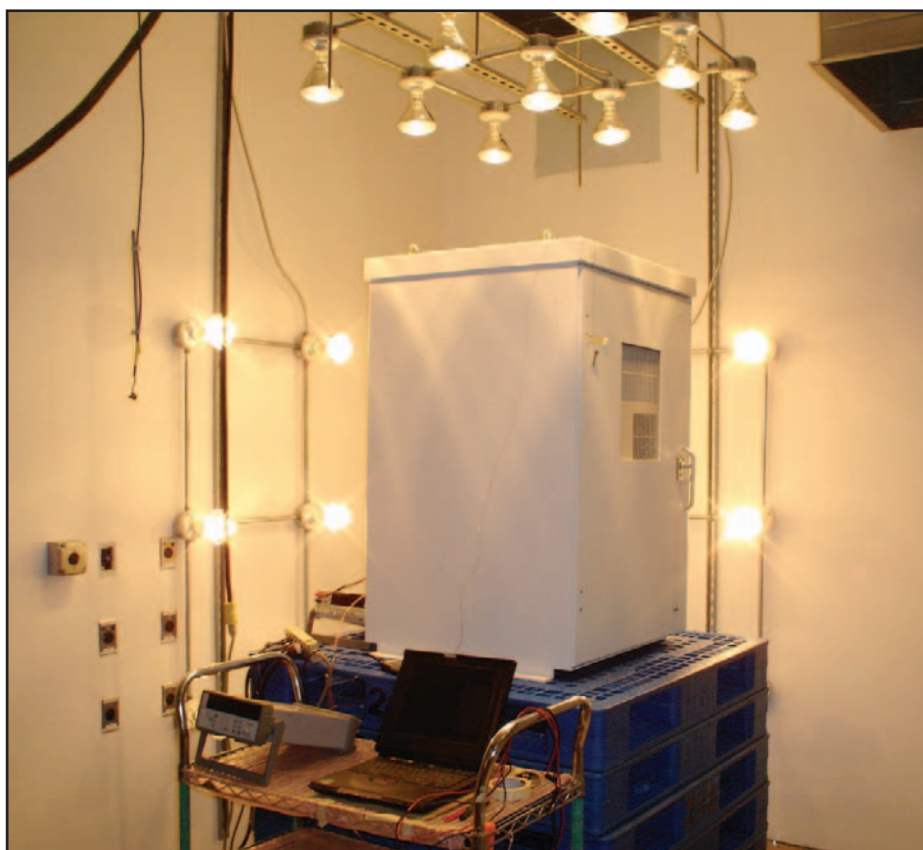
Figure 5: Solar loading test on system intended for outdoor installation
